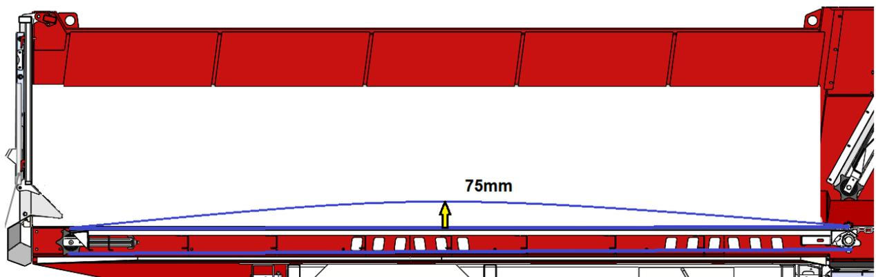
**CHECK ELEVATOR CHAIN TENSION.** Exert a pull at the mid-point of the elevator face. If necessary, adjust for approximately **35mm (1-1/2")** of movement from rest towards the rear of the wagon.
