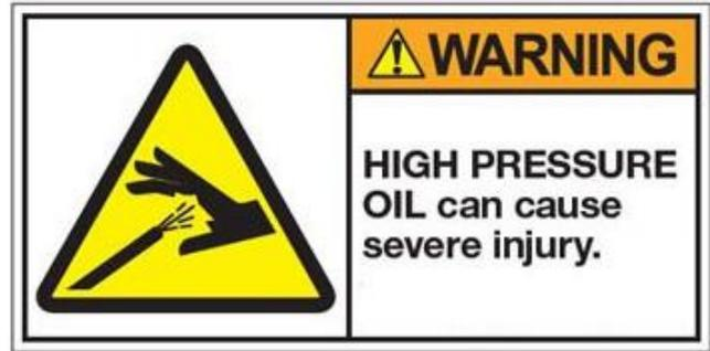
Never attempt to unblock equipment while it is still operating. Always disengage power take-off, hydraulics and shut down engine before removing materials, checking or servicing. Failure to follow these precautions is likely to result in serious injury.
