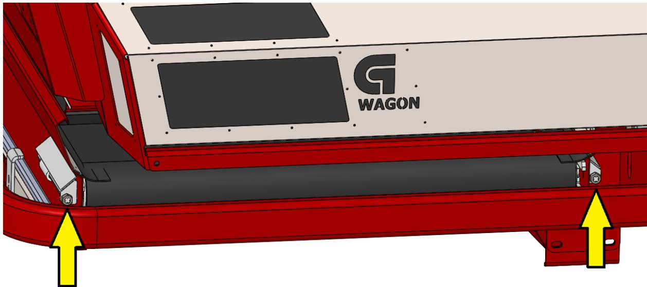
**All adjustments must be made with wagon running, preferably empty. Only adjust  $\frac{1}{4}$  of a turn at a time and run for at least 2 minutes between adjustments. THE BELT WILL RUN TO THE LOOSE SIDE.**
