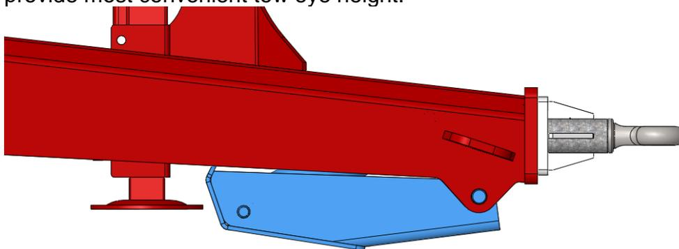
To operate, connect the two jack hydraulic hoses to the tractor. Standing away from the drawbar (in case of movement), turn the on/off lever to point along the hose (On position). The jack height may now be adjusted using the tractor hydraulics.
