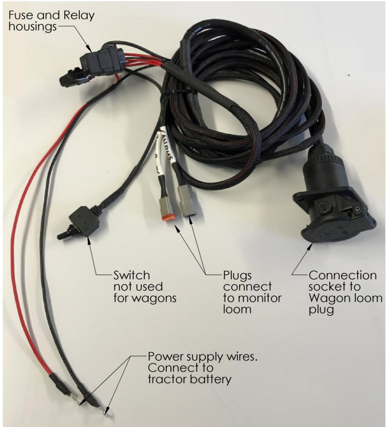
Connect Wagon loom plug to Tractor loom socket.
