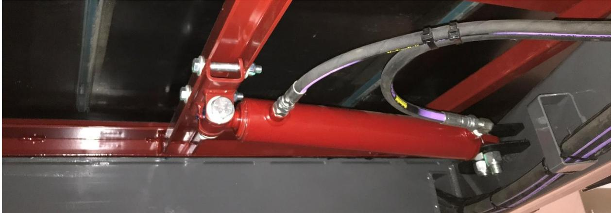
To operate, connect the two side shift hydraulic hoses to the tractor and adjust cross conveyor position using the tractor hydraulics.
