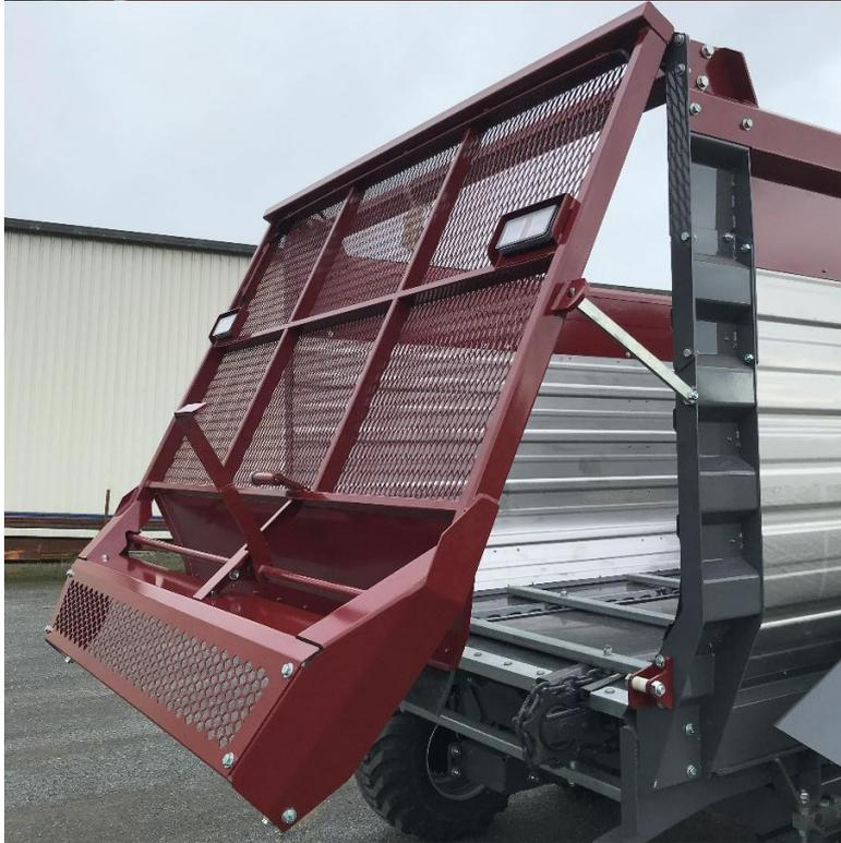
A stay is fitted which locates in the gate to hold it open for access.
