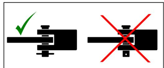
Always ensure when using a quick hitch that the locking tab has come out and is in the locked position before moving.
