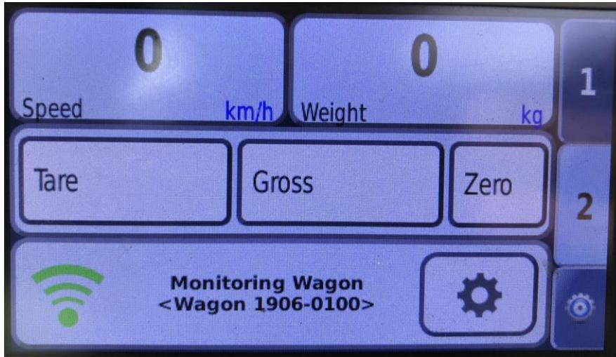
The wagon may now be loaded by the towing tractor, with live bin weight readout in the cab.
