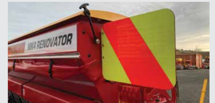
Transport visibility kit - Lights and high visibility boards for driving on the road
