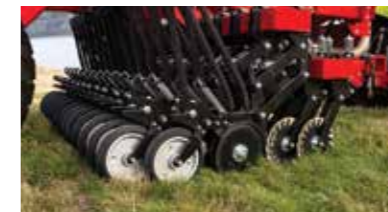
Opening Turbo Tilt disc, double discs on parallelogram & press wheels
