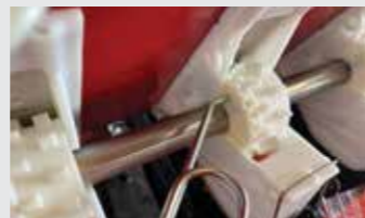
Dual large and fine metering wheels allow for a wide range of seed types and fertilisers
