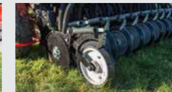
Press wheel following the double discs
