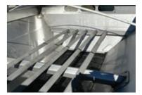
Weight reducing rail kit - reduces excessive weight / compaction on the belt during travelling
