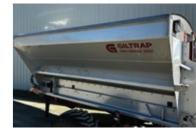
The 3mm grade 304 stainless steel bin provides years of corrosionfree use. The wide low profile bin is easy to fill and stable on steep hills
