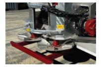
Independently touch screen adjusted spinners from the tractor seat with sectional boundary control spreading function
