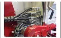
The proportional hydraulic control valve delivers oil to the belt drive and is adjusted automatically by the computer to maintain a constant fertiliser application rate
