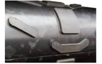
The extremely durable 850mm wide x 8mm thick vulcanised endless rubber belt, with 5mm chevron cleats, capably moves fertiliser, lime, compost and chicken manure efficiently through the rear door
