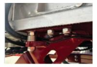
The stainless bin is bolted, not welded to the independent chassis. This makes it easy to remove and service if required, and minimises any risk of stress cracking from welding stainless to mild steel. Load cells for electronic weighing can be factory fitted or easily retro-fitted
